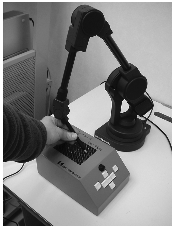
Photo 1. "Tactile Graphic Display with Pen Input Function" that allows drawing and erasing of figures any number of times by touching the figures real-time
