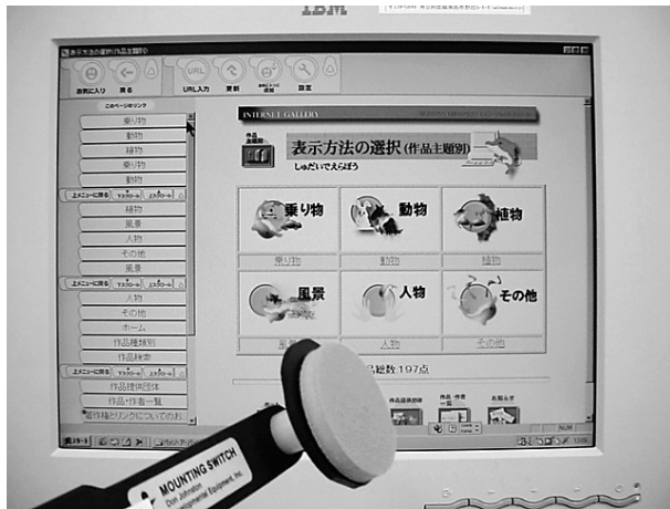
Photo 2. By means of its implemented step scan method, the Passo a Passo Browser allows one-switch users to browse web pages freely.
