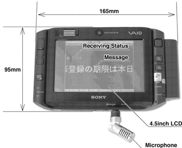
FIGURE 4. Appearance of the portable acoustic caption decoder (The sentence on the displays reads “The deadline of the registration is today...”)
